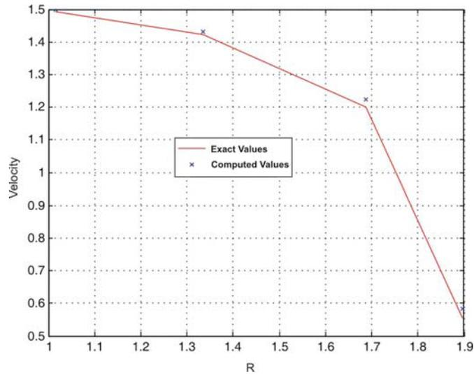
**Figure VI: Comparison of computed and analytical velocity distributions over the surface of an elliptic cylinder using 32 boundary elements with constant variation.**
