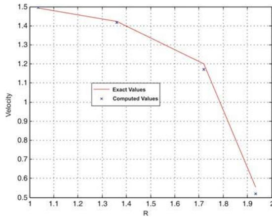
**Figure X: Comparison of computed and analytical velocity distributions over the surface of an elliptic cylinder using 32 boundary elements with linear variation.**
