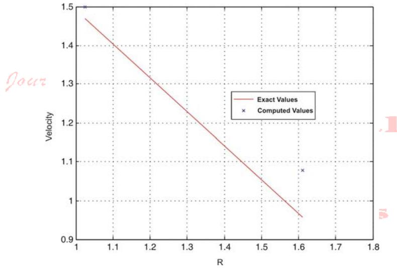
**Figure V: Comparison of computed and analytical velocity distributions over the surface of an elliptic cylinder using 16 boundary elements with constant variation.**
